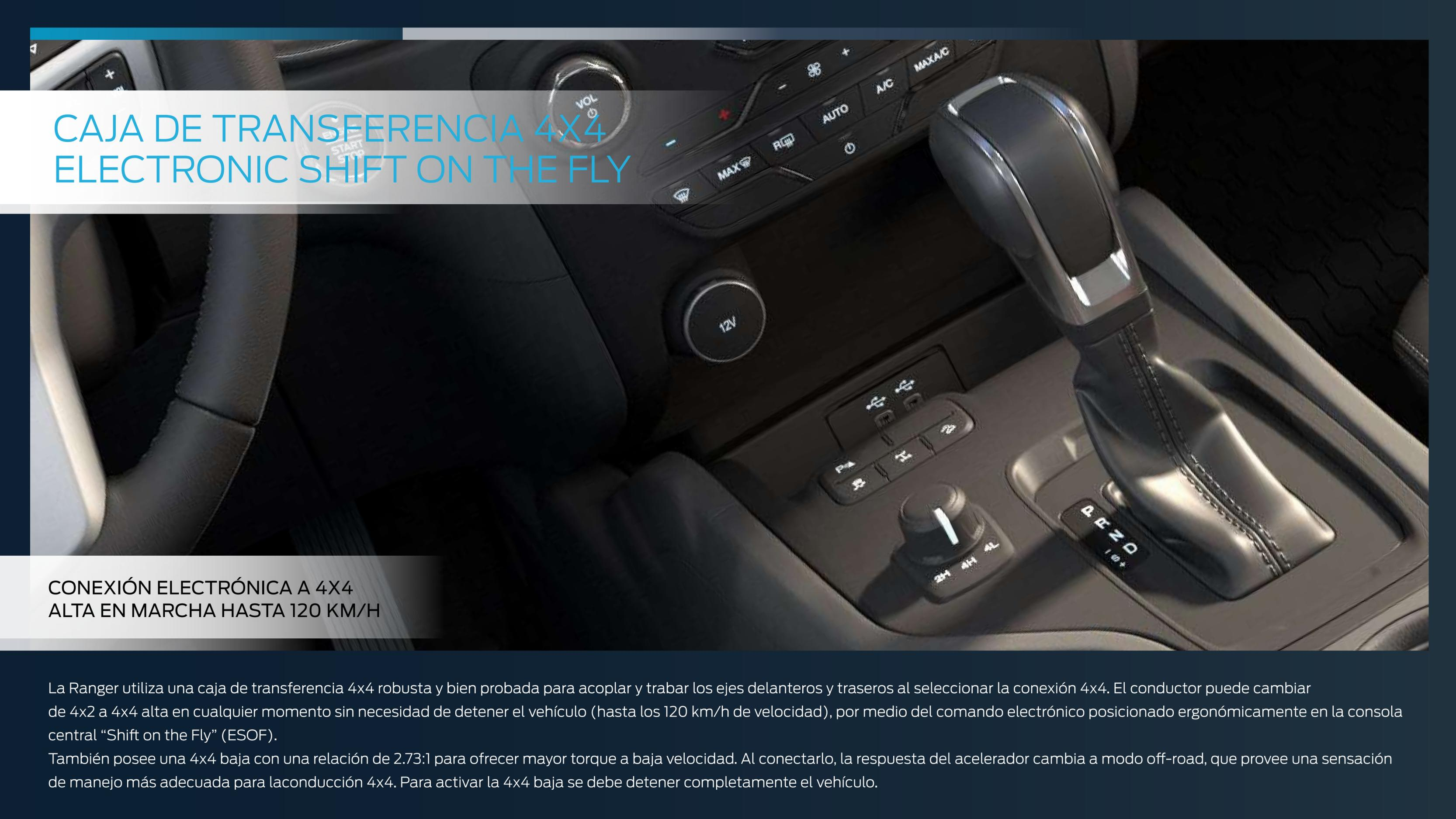
A close-up photograph of the center console of a vehicle. The focus is on the 4x4 electronic shift knob, which is a rotary dial with markings for 2H, 4H, and 4L. To its right is the gear shift lever with a leather-like grip and a 'P R N D' indicator. Above the shift knob are various climate and audio controls, including buttons for 'MAX', 'AUTO', 'A/C', and 'MAX A/C', and a '12V' power outlet. The background shows the steering wheel and dashboard area.
